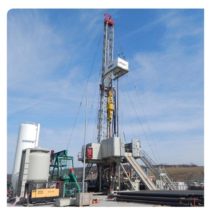
The rig MD150, produced by German manufacturer Streicher is of conventional design including several highend features. It is suitable for all workover operations and drilling operations with the advantage of fast rig moves,
