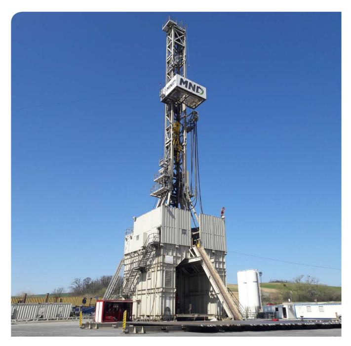
This new, modern land-drilling rig represents environmental and safety solutions as well as technological progress. The rig is designed and manufactured according to API 4F and the latest European regulations including low emissions and is fully ATEX certified. The rig is AC driven and joystick operated.
