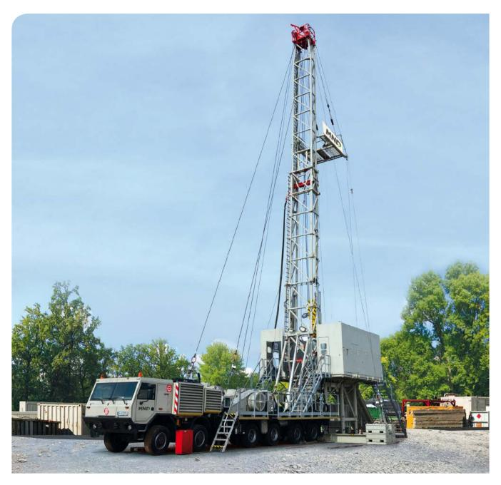
The rig MD80, produced by German manufacturer Streicher is of conventional design including several high-end features. It is suitable for all workover operations with the advantage of fast rig moves, easy operations and simple
